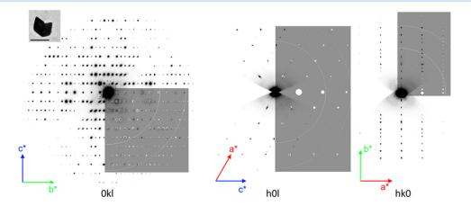
With the ELDICO ED-1 the experimental diffraction data show a perfect match with the simulated data
